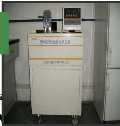
Low temperature embrittlement testing
